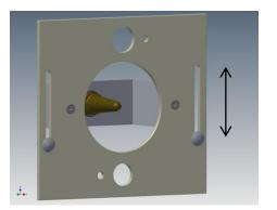
**Abb.7:** Front plate with teat at the teat bracket for already trained lambs and high position of the front plate
